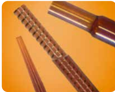
Polyimide with various controlled depth ablations
